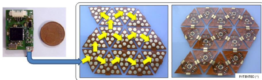
Figure 1 - The skin system. Triangular modules composed into networked patches.
