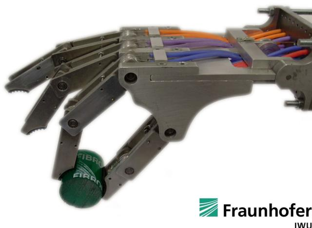
Figure - Gripping mechanism with self-sensing shape memory actuators
