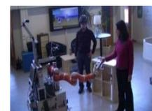
also to synthesize and perform a wide set of grasps, throughout the whole grasp taxonomy. A prototype of the DEXMART hand has been integrated on the COMAU Smart Six robot. This set-up is used for benchmarking the task **“Exchange of an object with human”**. To
